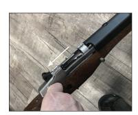
4. Invert the rifle so that the magazine well is facing up. Insert a ¼" steel rod, punch, screwdriver, or other suitable instrument into the hole in the rear of the trigger guard. Lift up, using the tool as a lever to spring open the trigger guard from its latched position.
