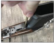
Remove the trigger housing assembly by carefully pulling it upward. Be careful not to damage the stock when removing or replacing the trigger housing.
