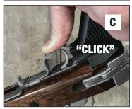
6. Cycle the slide handle and safety a few times to be certain the components are correctly assembled. Put the safety back "ON."
