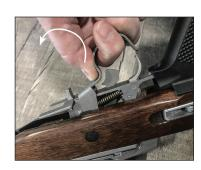
6. You can now remove the barrel/receiver assembly from the stock by lifting the rear of the assembly out of the stock and then pulling the stock rearward out of engagement with the gas block.
